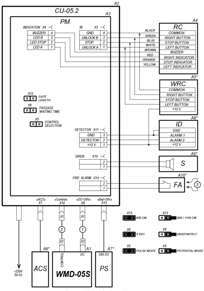
Figure 7 WMD-05S Wiring diagram
