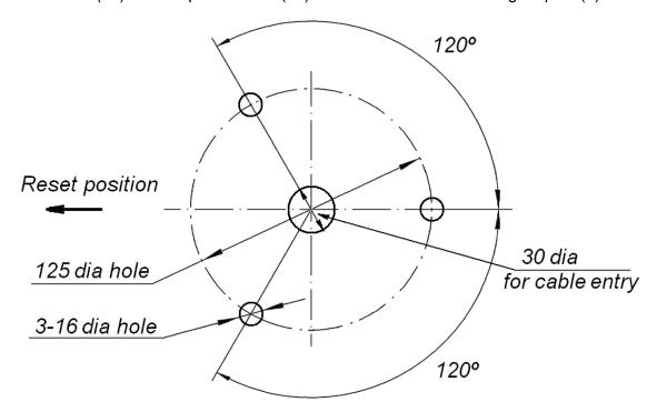
Figure 5 Mounting hole pattern
