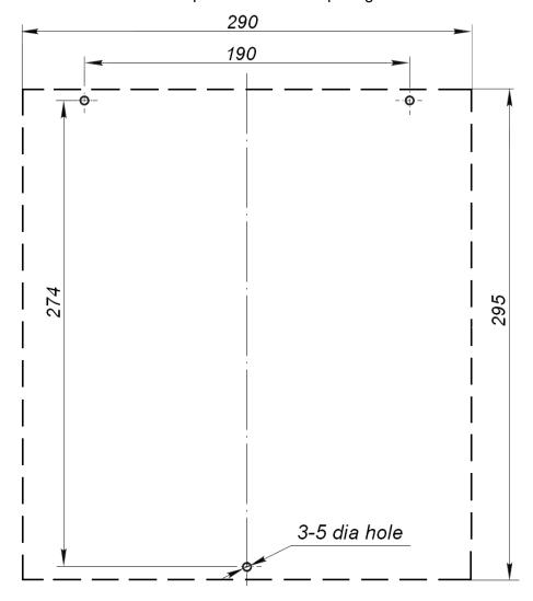
Figure 6 Hole pattern for the CU mounting
